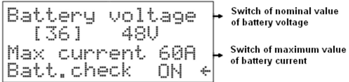
Fig. 3-3 Battery 1<sup>st</sup> screen.
